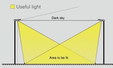
HiBoard LED Floodlight is specially designed for sports fields, minimizing loss of light and light pollution.
