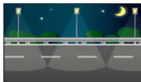
Light auto decrease to LOW DIM from a set time before midnight (VM-TB) to a set time after midnight (VM-TA)
