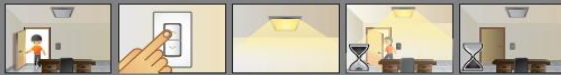
Occupant presence Light is off Press button Light on Occupant leave - Delay time start Light remains on Delay time end Light auto off
