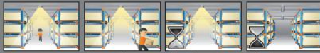
Occupant presence Light auto on Occupant leave Light remains on Delay time start Light remains on Delay time end Light auto off
